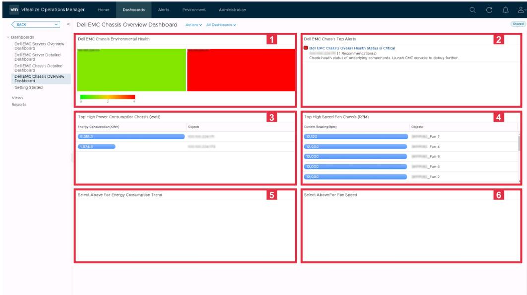
Figure 3. Dell EMC Chassis Overview Dashboard
